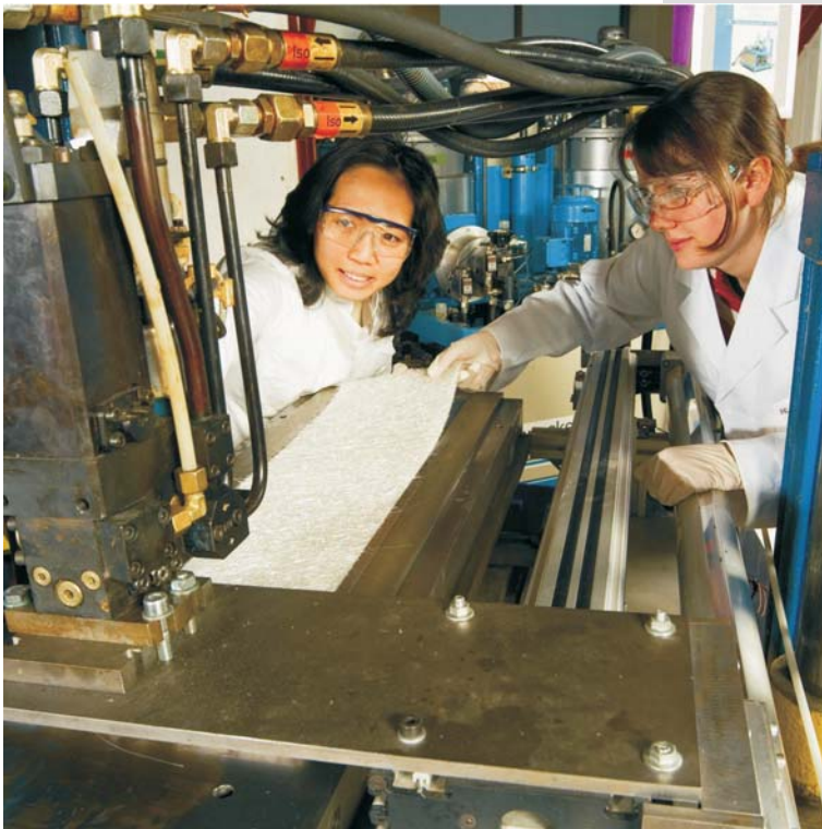
The PU laboratory (top) An open-mould S-RIM process (bottom)
