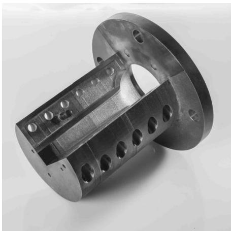
Additively manufactured demonstrator die (Photo: IKV/Fröls)
